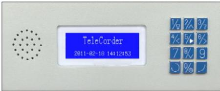
Front with speaker, LCD display, & keypad
