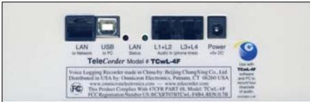
Back with input and output connections
