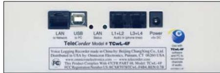
Back with input and output connections
