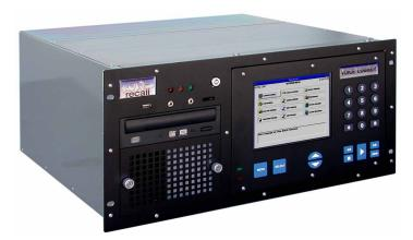
Total Recall Max is the premium VoIP call recording solution for enterprise-critical applications. Mirrored hard-drive storage and a hot-swap power supply are standard features, ensuring the integrity of your recording solution in the most demanding conditions. Total Recall Max utilises the latest Intel Core 2 Duo processors, for maximum speed and reliability.
