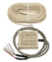
**RSA-M4** Two-way radio adapter with a relay that switches between receive and transmit audio. Similar to RSA-M3, the RSA-M4 has a relay that connects to 12vDC transmitter power and an audio transformer to boost the volume of transmitter audio that is fed to the recorder. The relay is used to switch its audio output jack from receive audio to transmit audio only when the radio is transmitting.
