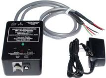
**RSA-U5** Two-way radio adapter with active amplifiers and optically isolated PTT sensing. Similar to RSA-M4, the RSA-U5 has screwdriver adjustable amplifiers to boost weak receiver and transmitter audio levels and a low power optically sensing circuit to mute microphone audio when the radio is not transmitting. Includes AC power adapter.
