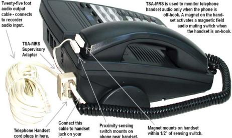
TSA-MRS Telephone handset supervisory adapter — with proximity switch audio muting. The TSA-MRS has a small proximity sensing magnetic reed switch that is used to mute handset audio when a small magnet (mounts on the handset of your phone) is within 1/2" of the sensing switch that mounts on your phone. Used in rare cases where handset audio is not muted when your phone is hung-up and the standard TSA-3LM cannot be used satisfactorily.
