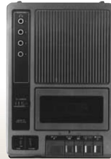
The VP series of cassette tape players is designed to play back the recordings made on the VLR series of OMNICRON professional Voice Logging Recorders. It provides an inexpensive means of playing tapes without tying up the main recorder/player. Since these players do not have the ability to make recordings, accidental erasure is not possible.
