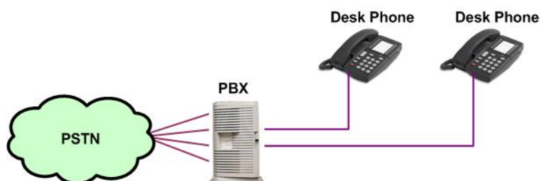
Figure 2: Analogue Telephone Connections (before)
